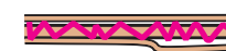
Forbidden route drawn irregularly, gives appearance of crossing points. Obscures adjacent permitted route
