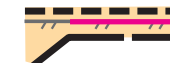
Solid straight line as uncrossable boundary, can appear as symbol 843, causing confusion
